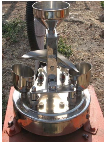
Figure 6: Tipping Bucket Rain Gauge
