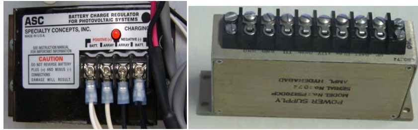
Fig. 6.1 Sutron (left) and Astra(right) solar charge regulators
